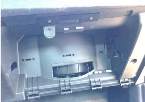
New latch attached
