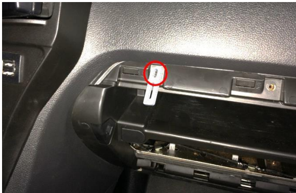
Cable retaining bracket installation
